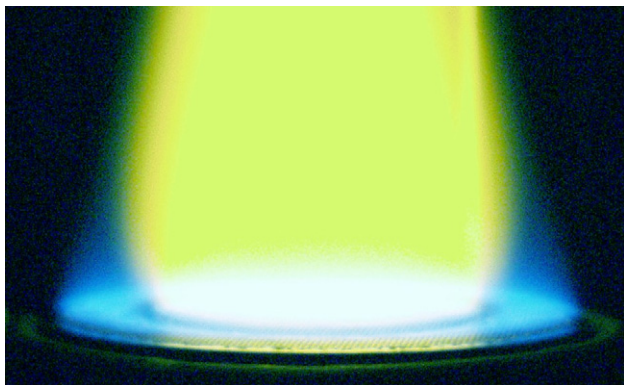
Figure 2. Photograph of the model flat burner operating on \text{CH}_4/\text{air} at the stoichiometric ratio. Central flow: Na-seeded, co-flow: unseeded.
