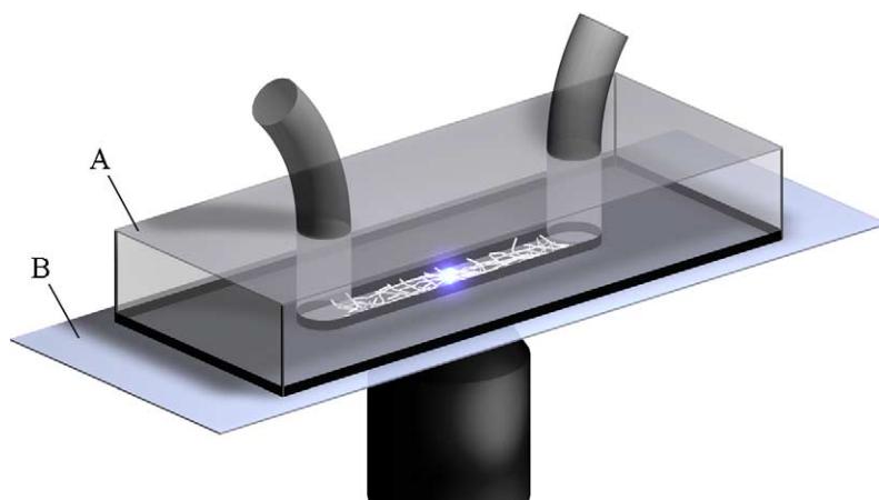
Fig. 1. Micro flow cell consisting of a PMMA block (A) with entry and exit holes and a channel milled at its base. Heat-bonded PET fibres at a bulk voidage of 95% are placed in the channel and a glass cover slip (B) is attached to the bottom of the PMMA block using double-sided sellotape. Biomass suspension is dispensed by a syringe pump and particle capture takes place in the flow cell fibre network. Biomass detachment is achieved using a fluid oscillator connected to the inlet of the flow cell. The laser scanning confocal fluorescence microscope, located beneath the flow cell, directly images both these processes.
