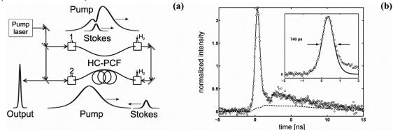
**Fig. 1 (a)**: Sketch of the set-up for generation of sub-ns pulses by BSRS; **(b)** Temporal structure of the input (seed) Stokes pulse (dashed line) and the output amplified Stokes pulse (circles) measured after a 4 m-long HC-PCF filled with hydrogen at p=1.5 bar. The inset shows a fit of the Stokes pulse envelope to the sech<sup>2</sup>(x) function predicted by theory; the agreement is excellent.
