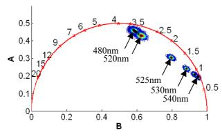
In the literature there are few examples of excitation wavelength resolved confocal microscopy and particular in FLIM applications, because suitable light sources have not been available. Here, we report on the combined application of fluorescence excitation spectral scanning with lifetime imaging. Fluorescence decays were sampled for each excitation wavelength with Time Correlated Single Photon Counting (TCSPC), through use of a pulsed, fibre laser
