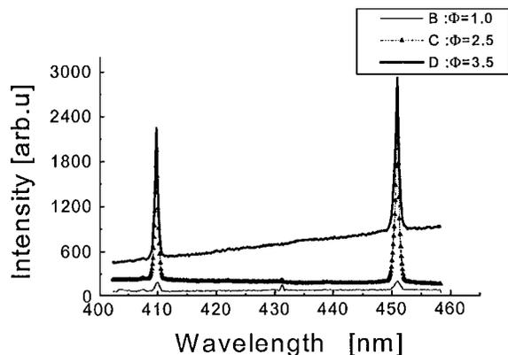
Fig. 2. Emission spectra from three  $C_2H_2$  flames seeded with the same indium concentration, collected through a spectrometer. The detected indium emission increases with  $\Phi$ . The increasing background originated from the soot particle emission.
