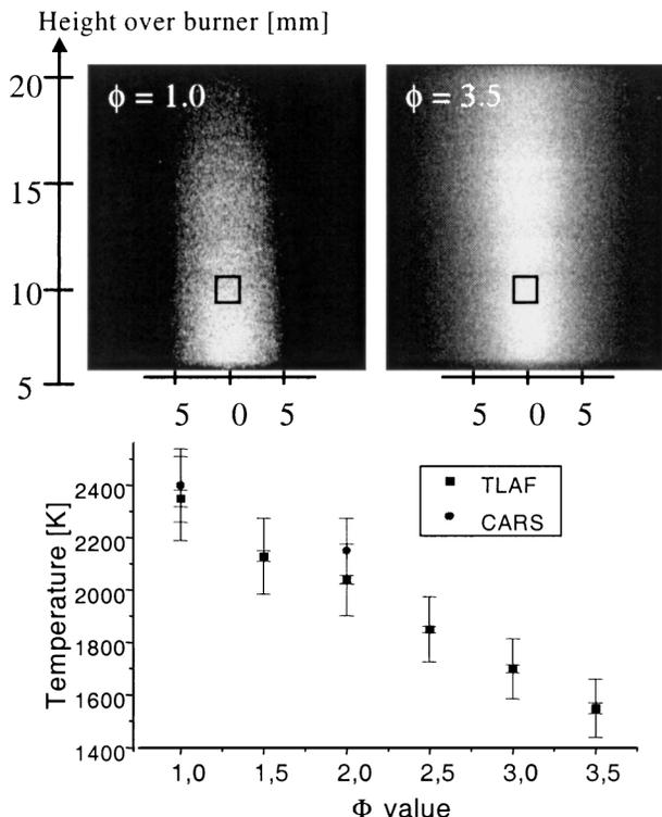
Fig. 3. Mean TLAF temperatures and two CARS reference temperatures for several  $\Phi$  values in a  $C_2H_2$ /air flame (bottom). Top, the 410-nm TLAF signals for  $\Phi = 1$  and  $\Phi = 3.5$ . The temperatures were calculated in the regions indicated by the rectangles shown in the fluorescence images.
