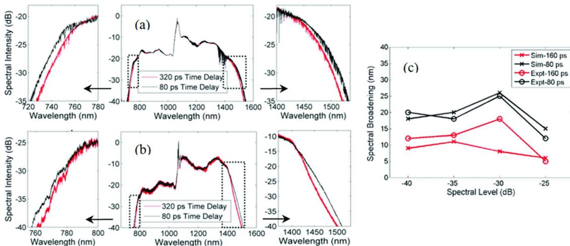
Fig. 3. (Color online) (a) Experimental and (b) simulated double input pulse SC spectra. (c) The spectral broadening of pulse pairs at initial separations of 160 and 80 ps is compared with effectively independent pulses at 320 ps separation, for experimental measurements and time-aliased predictions. The experimental spectral features around 1350 to 1400 nm are due to ambient water vapor absorption.
