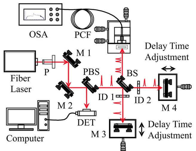
Fig. 2. (Color online) Experimental setup for double pump-pulse SC generation: P, polarizer; M, mirror; ID, iris diaphragm; BS, 50% beam splitter; PBS, 8% pellicle beam splitter; DET, light detector; and OSA, optical spectrum analyzer.
