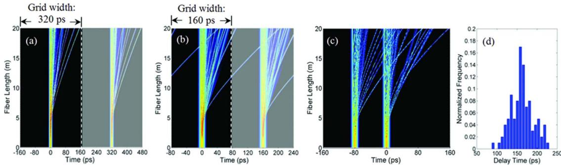
Fig. 1. (Color online) SC simulations using (a) a 320 ps time grid and (b) a 160 ps time grid, resulting in pulse wraparound and associated extrasoliton collisions after 17 m. Copies of the simulation grid (gray area) illustrate the physical interpretation of time-aliased simulations. (c) A full simulation of a pair of pulses. (d) Histogram of maximal soliton delays in 150 simulations using 320 ps grids, as depicted in (a).
