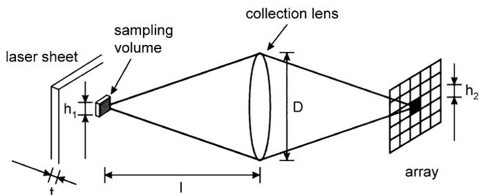
**Fig. 3.** LIF signal collection from a laser sheet. The magnification is  $M = h_2/h_1$ , the sheet thickness is given by  $t$ , the collection  $f$ -number is given by  $f_{\#} = D/l$ .
