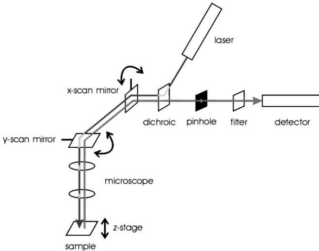
**Fig. 4.** Principle of confocal laser scanning fluorescence microscopy.
