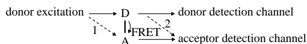
Figure 1. Crosstalk in sensitized emission FRET measurements. With no crosstalk (paths 1 and 2 inactive), the only path to the acceptor channel is via FRET. When crosstalk is present (paths 1 and 2 active), contamination of the FRET signal occurs.
