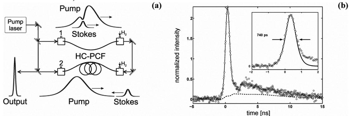
**Fig. 1 (a):** Sketch of the set-up for generation of sub-ns pulses by BSRS; **(b)** Temporal structure of the input (seed) Stokes pulse (dashed line) and the output amplified Stokes pulse (circles) measured after a 4 m-long HC-PCF filled with hydrogen at  $p=1.5$  bar. The inset shows a fit of the Stokes pulse envelope to the  $\text{sech}^2(x)$  function predicted by theory; the agreement is excellent.
