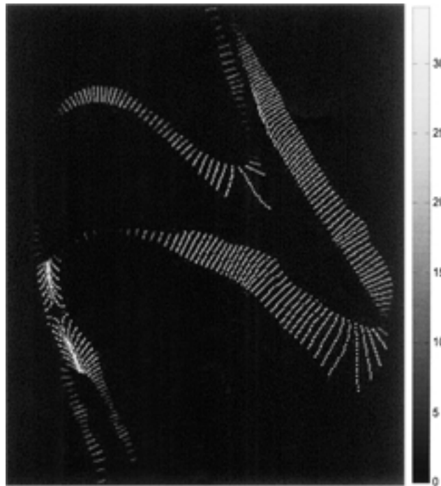
Figure 13. Flame front velocities estimated from the OH-PLIF image sequence shown in Fig. 8 (frames b and c). The color-bar to the right shows the velocity values in m/s.
