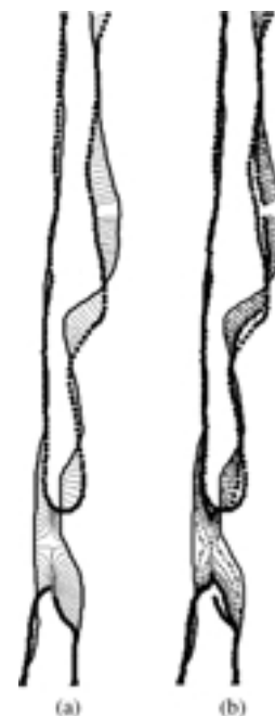
Figure 18. Curve matching of flame fronts extracted from Fig. 17(b) and (c). (a) Matching paths. (b) Interpolated curves (gray colors) between the original flame fronts (black).
