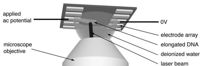
FIG. 2. Schematic diagram of the experimental arrangement.
